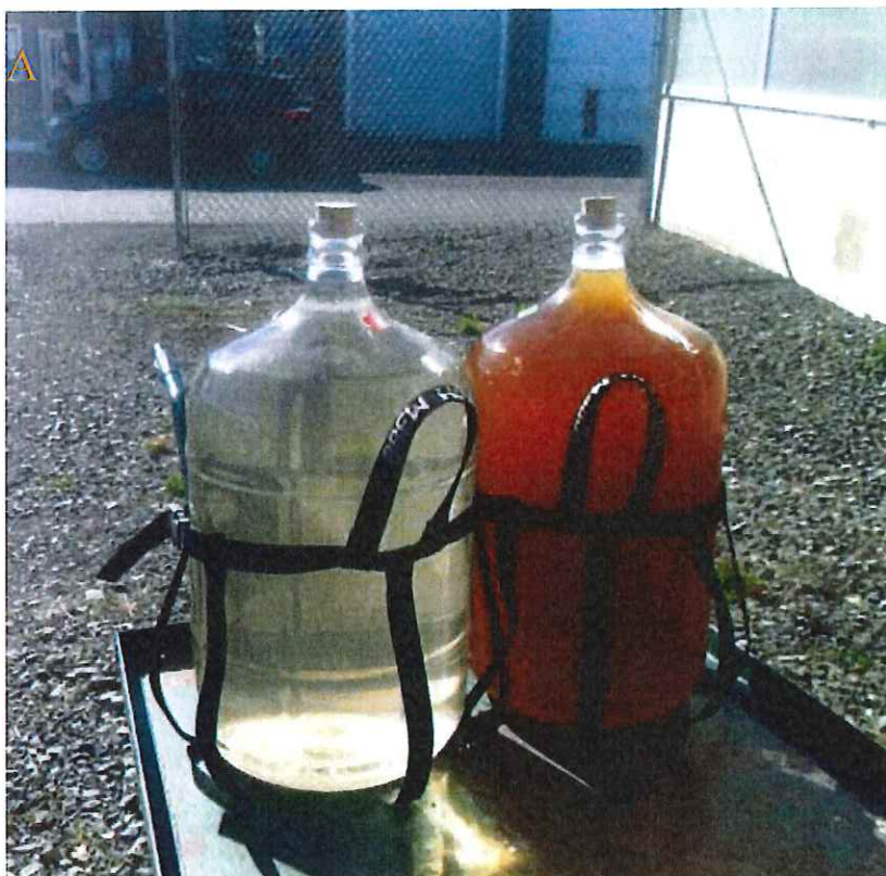
Figure 8. Samples of “unfiltered” (clearer liquid) runoff and runoff “filtered” (brownish liquid) through a sand-organic matter bioretention system. Photo from a presentation by J. McIntyre. Used with permission.
