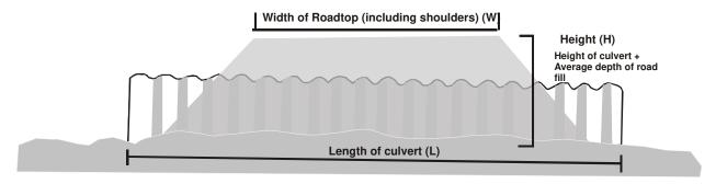
Determining the length of a culvert:
