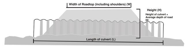
Determining the length of a culvert:
