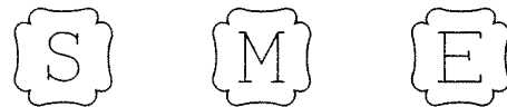
FIG. PG-105.1 OFFICIAL SYMBOLS FOR STAMPS TO DENOTE THE AMERICAN SOCIETY OF MECHANICAL ENGINEERS' STANDARD FOR BOILERS
