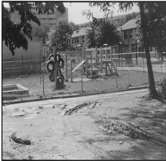
Figure 11.21b Fencing as an Interim Control for Bare Soil Hazards.
