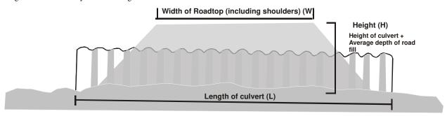
Determining the length of a culvert:
