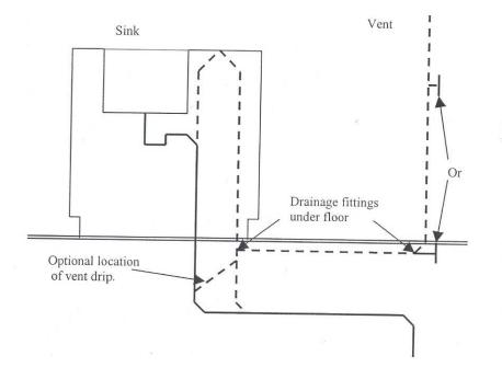
Cleanout is required for horizontal vent pipe under floor.
