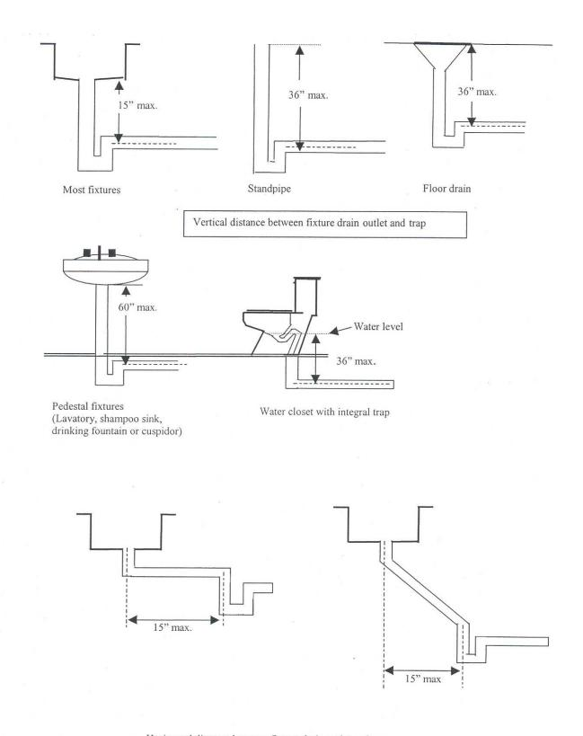
Horizontal distance between fixture drain outlet and trap
