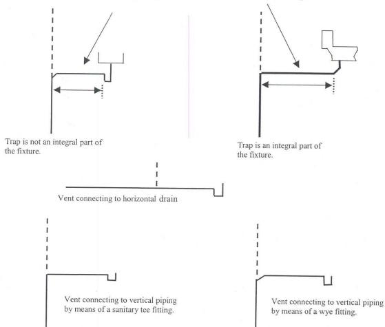
Developed length of fixture drain between the vent and trap.
