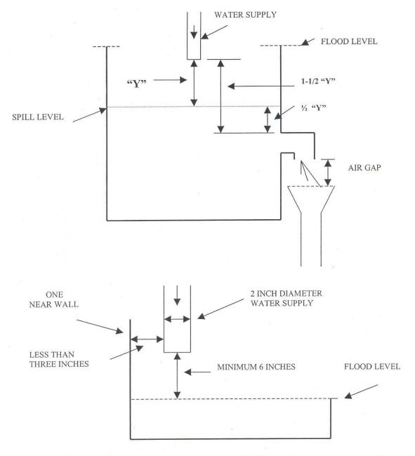
If distance is three times or greater than the diameter of water supply (2 inches) then the air gap is two times the diameter of the water supply, (i.e.,  $2 \ge 2 = 4$  inches)
