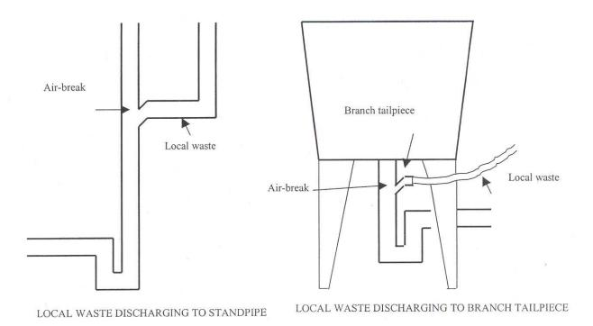
A-82.33 (8) (d)-1. LOCAL WASTE PIPING SERVING WATER HEATER TEMPERATURE AND PRESSURE RELIEF VALVES.
