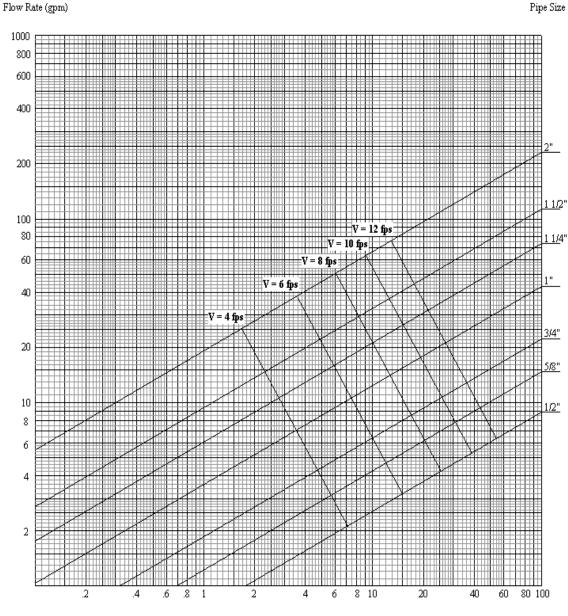
Pressure loss due to friction (psi/100 ft of pipe)
