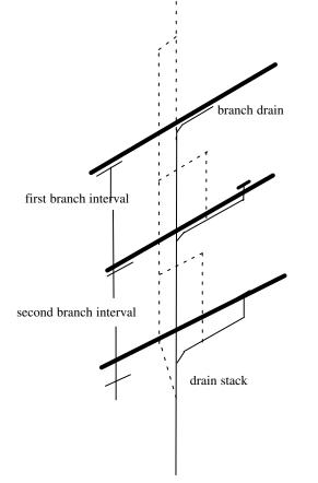
A-82.31 (4)-2. INSTALLATION OF VENT STACK AND STACK VENT.
