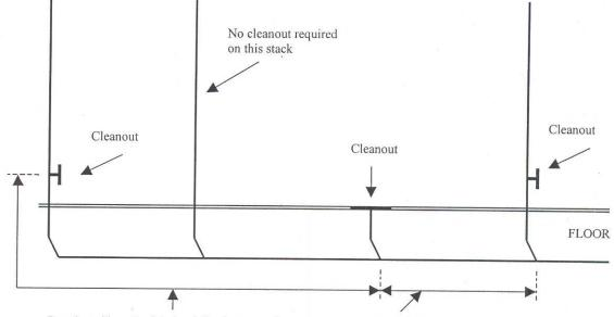
Developed length of drain piping between cleanouts not exceeding 75 feet.
