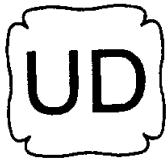
FIG. UG-129.2 OFFICIAL SYMBOL FOR STAMP TO DENOTE THE AMERICAN SOCIETY OF MECHANICAL ENGINEERS' STANDARD FOR RUPTURE DISK DEVICES
