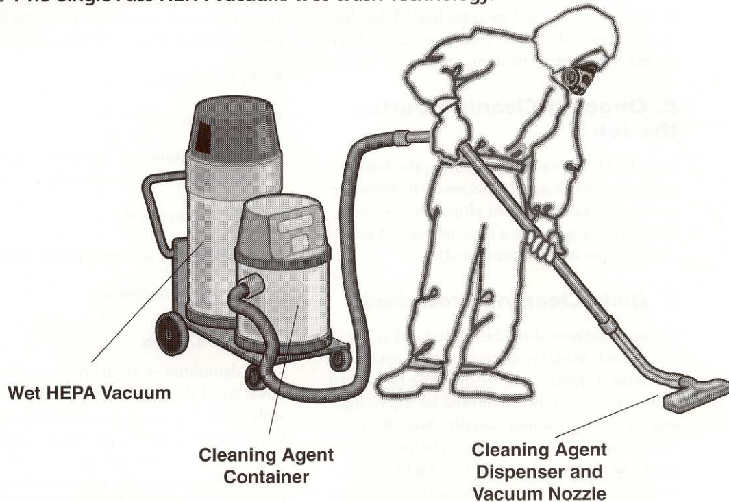
Figure 14.5 Single-Pass HEPA Vacuum/Wet Wash Technology.
