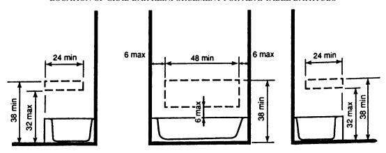
NOTE: The areas outlined in dashed lines represent locations for future installation of grab bars for typical fixture configurations.
