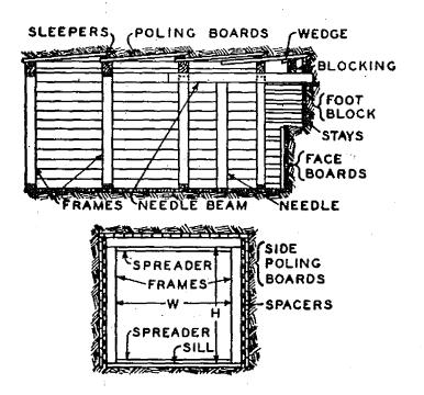
Fig. 11.—Poling Board Method of Timbering.
