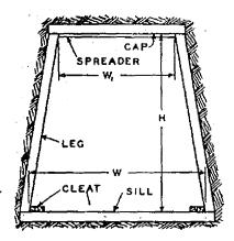
Fig. 7.—Modified Box Type of Timbering.
