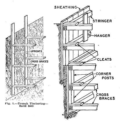
Fig. 2.—Trench Timbering— Loose Soil
