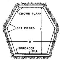
Fig. 9.-Modified Hexagonal Type of Timbering.
