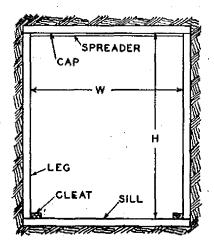
Fig. 5.—Box Type of Timbering.
