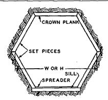
Fig. 8.—Hexagonal Type of Timbering.
