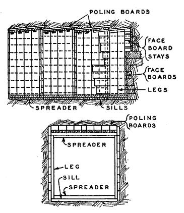
Fig. 12.—Poling Board Method of Timbering.
