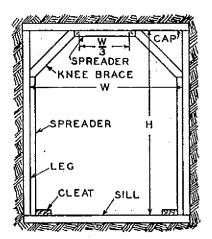
Fig. 6.—Box Type of Timbering.
