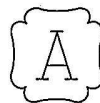
FIG. PG-105.3 OFFICIAL SYMBOL FOR STAMP TO DENOTE THE AMERICAN SOCIETY OF MECHANICAL ENGINEERS' STANDARD FOR WELDED PIPING
