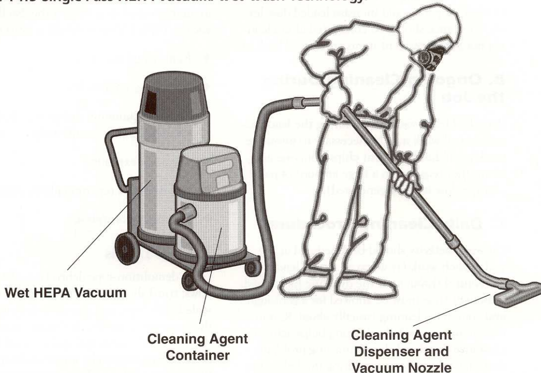
Figure 14.5 Single-Pass HEPA Vacuum/Wet Wash Technology.
