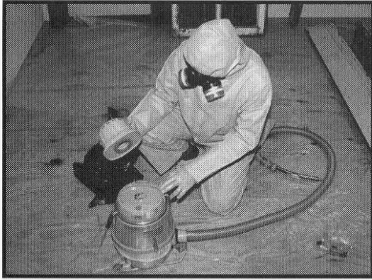
Figure 11.16f Remove and Replace HEPA Filter Assembly.
