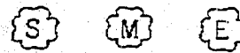
FIG. PG-105.1 OFFICIAL SYMBOLS FOR STAMPS TO DENOTE THE AMERICAN SOCIETY OF MECHANICAL ENGINEERS' STANDARD FOR BOILERS
