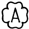
FIG. PG-105.2 OFFICIAL SYMBOL FOR STAMP TO DENOTE THE AMERICAN SOCIETY OF MECHANICAL ENGINEERS' STANDARD FOR ASSEMBLY
