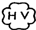
FIG. HG-402 OFFICIAL SYMBOL FOR STAMP TO DENOTE THE AMERICAN SOCIETY OF MECHANICAL ENGINEERS' STANDARD
