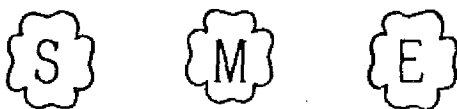
FIG. PG-105.1 OFFICIAL SYMBOLS FOR STAMPS TO DENOTE THE AMERICAN SOCIETY OF MECHANICAL ENGINEERS' STANDARD FOR BOILERS
