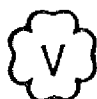
FIG. PG-105.4 OFFICIAL SYMBOL FOR STAMP TO DENOTE THE AMERICAN SOCIETY OF MECHANICAL ENGINEERS' STANDARD FOR SAFETY VALVES
