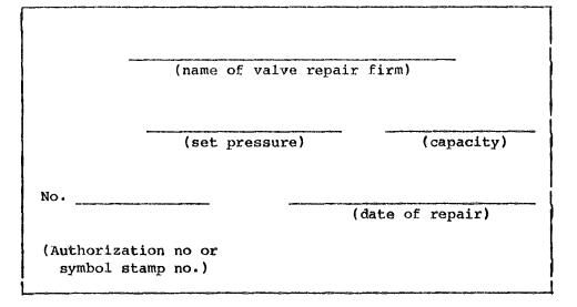
Figure 41.07 VALVE REPAIR NAMEPLATE
