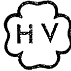
FIG. HG-402 OFFICIAL SYMBOL FOR STAMP TO DENOTE THE AMERICAN SOCIETY OF MECHANICAL ENGINEERS' STANDARD
