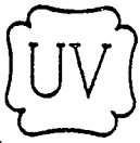
FIG. UG-129 OFFICIAL SYMBOL FOR STAMP TO DENOTE THE AMERICAN SOCIETY OF MECHANICAL ENGINEERS' STANDARD
