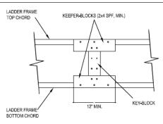
Detail 2: Attachment of Deck Ledger to Floor System with MPCW Trusses, When Ledger is Installed Parallel to Truss Span & Spacing of Screws is Less Than the Spacing of the Verticals
