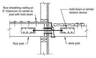
**Hold-down tension devices.** Hold-down tension devices, if used instead of perpendicular bracing as described above, must be provided in at least two locations per deck, and each device must have an allowable-stress-design capacity of at least 1,500 pounds.
