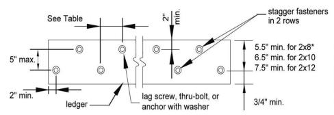
See Figure 11 for band-board fastener spacing.
