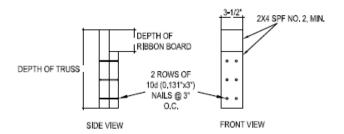
ATTACH TOP OF KEY-BLOCK TO INSIDE FACE OF RIBBON BOARD WITH 2 - 10d (0.131" x 3") THROUGH NAILS AND 2 - 10d TOE-NAILS. ATTACH BOTTOM OF KEY-BLOCK TO SILL PLATE WITH 4 - 10d TOE-NAILS
