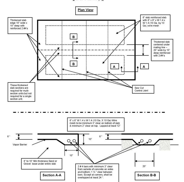
Note: Perimeter insulation is NOT required.
