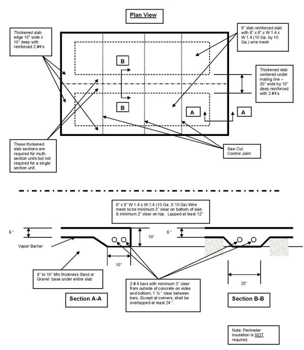
Acceptable slab on grade for pier supported manufactured home produced on or after April 1, 2007 [per SPS 321.40 (1)]
