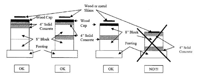
(p) *Footings and foundations*. This is a department requirement in addition to the requirements in 24 CFR 3285.301: Footings and foundations may be designed in accordance with any of the following:
