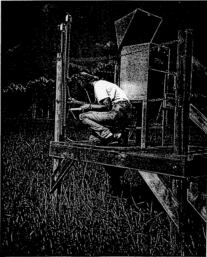
Air monitoring stations will continuously measure air quality in the area to make sure the mine meets all air standards.
